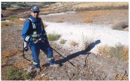
Photo 6. Surface Methane Concentration Scan Using a Portable FID Instrument
