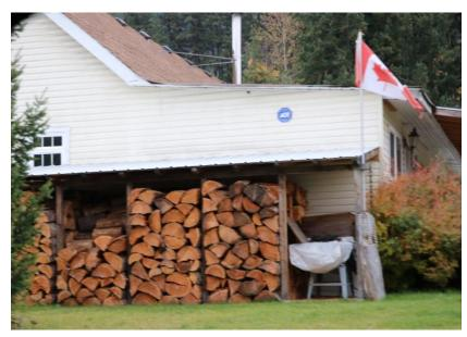
Figure 10 Ignition of outbuildings with 15m of a home pose a significant risk to home ignition due to prolonged exposure to extreme radiant heat
