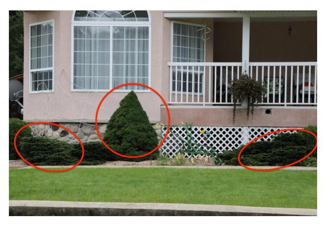
Figure 9 The presence of nearby combustible debris (such as wood pallets, ladders, building materials etc.) and combustible plants pose a high risk to ignition of a building's exterior.
