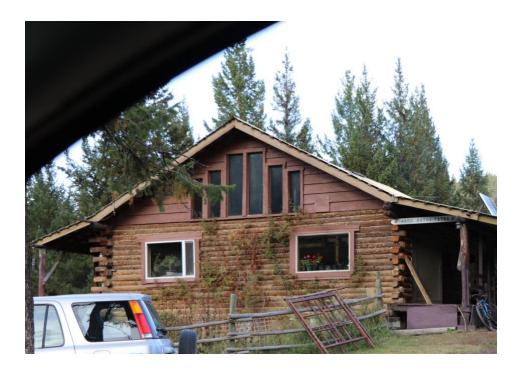
Figure 9 The presence of nearby combustible debris (such as wood pallets, ladders, building materials etc.) and combustible plants pose a high risk to ignition of a building's exterior. Climbing vines — as seen in the photo — pose a risk for vertical fire growth along the building's exterior.
