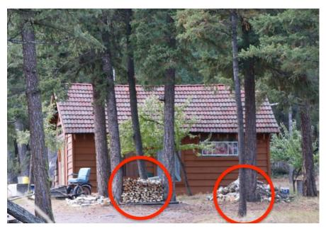
Figure 10 Firewood is a risk for home ignition when found within 10m of a structure. This is because of its easy ignitability and ability to sustain high radiant heat for a length of time.
