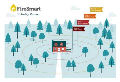
Figure 2 FireSmart Canada utilizes the concept of priority zones surrounding a home to help residents prioritize their hazard reduction efforts. A home's immediate surroundings (Zones 1 and 1a) are of immediate concern to the homeowner and should be targeted aggressively to reduce ignition hazards to the home.
