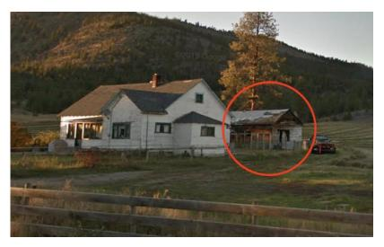
Figure 10 Ignition of outbuildings with 15m of a home pose a significant risk to home ignition due to prolonged exposure to extreme radiant heat
