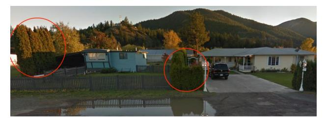
Figure 9 The presence of nearby combustible debris (such as wood pallets, ladders, building materials etc.) and combustible plants pose a high risk to ignition of a building's exterior.
