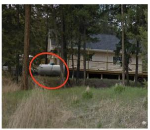
Figure 11 Propane tanks should be relocated 10m away from a home if possible. There should be a 3m fuel free zone established and relief valves should be tested for functionality and aimed away from structures
