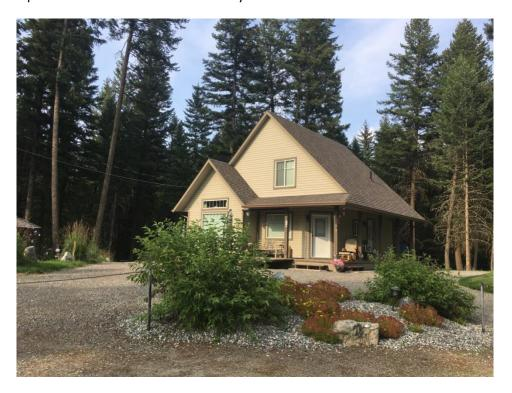
Figure 14 This home demonstrates several FireSmart landscaping attributes. The gravel provides a non-combustible surface creating a break from direct flame contact to the home. Conifers have been removed up to 10m away and ladder fuels have been cleared. Leafy, deciduous plants are the preferred vegetation to be found in zone 1.
