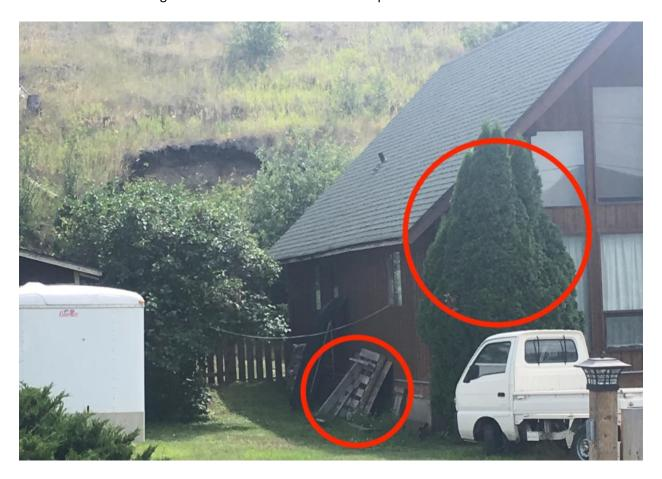
Figure 8 The presence of nearby combustible debris (such as wood pallets, ladders, building materials etc.) and combustible plants pose a high risk to ignition of a building's exterior. (photo not taken from Iron Mountain)
