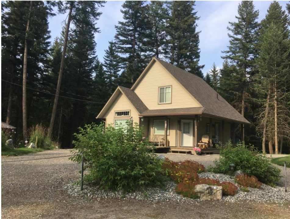
Figure 11 This home demonstrates several FireSmart landscaping attributes. The gravel provides a non-combustible surface creating a break from direct flame contact to the home. Conifers have been removed up to 10m away and ladder fuels have been cleared. Leafy, deciduous plants are the preferred vegetation to be found in zone 1.
