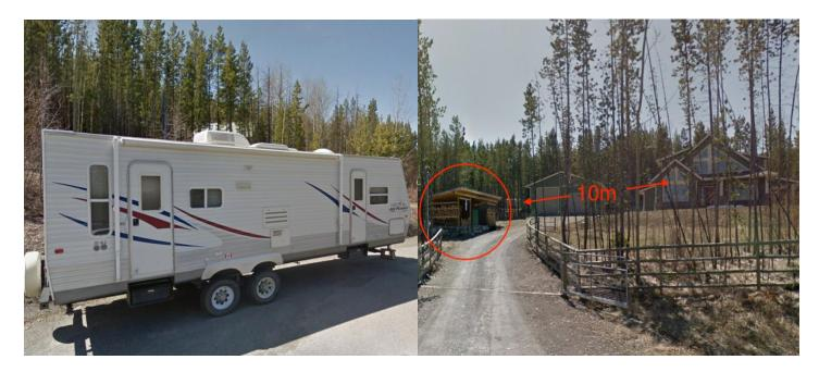
Figure 9 Combustibles such as firewood and other personal items (i.e. campers, trailers, RVs, etc.) should be stored 10m away from the home
