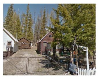
Figure 10 Conifers within 10m of the home pose a significant risk towards home ignition. This is due to the relative ease of ignition and ease of fire transference from the ground to aerial fuels, creating increased fire intensities.
