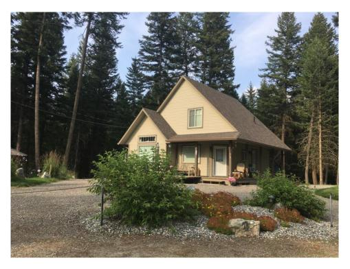
Figure 13 This home demonstrates several FireSmart landscaping attributes. The gravel provides a non-combustible surface creating a break from direct flame contact to the home. Conifers have been removed up to 10m away and ladder fuels have been cleared. Leafy, deciduous plants are the preferred vegetation to be found in zone 1.
