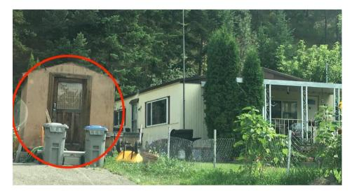
Figure 8 Ignition of outbuildings with 15m of a home pose a significant risk to home ignition due to prolonged exposure to extreme radiant heat
