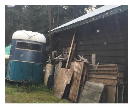
Figure 10 Combustible materials stacked along a structure pose a threat to home ignition
