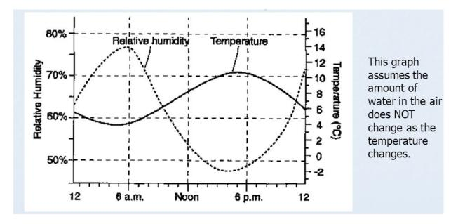
Figure 4 shows the relationship between temperature and relative humidity, as temperatures increase and the overall water content in the air does not change, relative humidity decreases. This affects fire behavior through the increased drying of fuels
