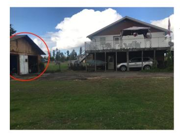
Figure 8 Nearby buildings are a potential fuel source. Any structure within 15m of the home should have FireSmart principles applied to mitigate ignition
