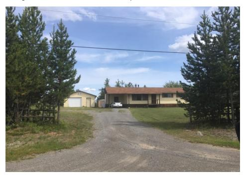
Figure 7 Burning combustibles against a home increases the risk of home ignition as the heat/flame challenges the exterior material's resiliency. As pictured, homes should be free of combustible plants and materials within Zone 1a (0-1.5m), also known as the "non-combustible zone".
