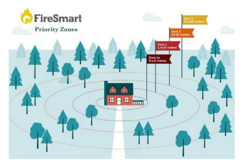
Figure 2 FireSmart Canada utilizes the concept of priority zones surrounding a home to help residents prioritize their hazard reduction efforts. A home's immediate surroundings (Zones 1 and 1a) are of immediate concern to the homeowner and should be targeted aggressively to reduce ignition hazards to the home.
