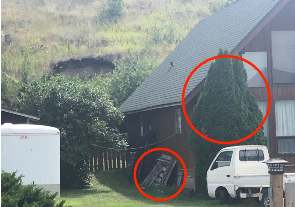
Figure 7 The presence of nearby combustible debris (such as wood pallets, ladders, building materials etc.) and combustible plants pose a high risk to ignition of a building's exterior (photo not taken from Blackpool)
