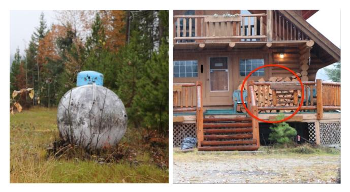
Figure 9 Both propane and firewood pose significant risk to home ignition during wildfire event when they're found within 10m of a home. As well, they're more likely to ignite when in contact with vegetation. By establishing fuel free zones homeowners can mitigate this risk.
