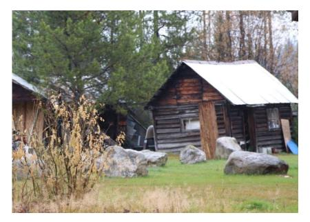
Figure 8 Ignition of outbuildings with 15m of a home pose a significant risk to home ignition due to prolonged exposure to extreme radiant heat
