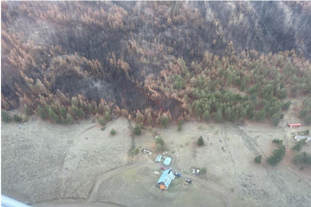
Photo D-29 Aerial overview photo of 5028 Venables Valley Rd (center) and element A6 (right). Note the evidence of overland flow left of 5028 Venables Valley Rd and between 5028 Venables Valley Rd and element A6. Photo taken by BGC on November 18, 2024.
